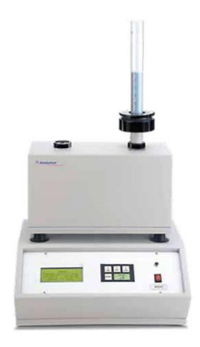
Tap Density Test Apparatus is designed for determination of the tapped density of powder samples by tapping the cylinder under specific conditions. It can also be used for Granules, Flakes etc.
